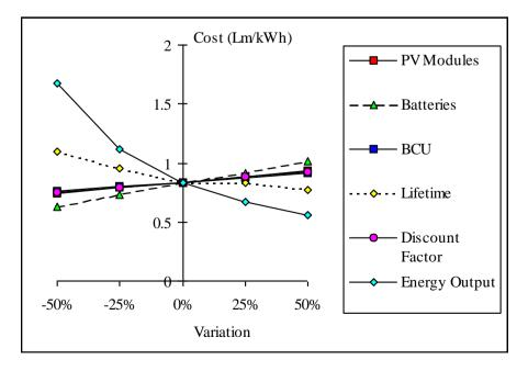
FIGURE 3: Spider diagram of the variable parameters used in the life cycle costing.
