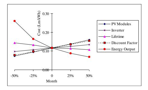
FIGURE 4: Spider diagram of the varied parameters involved in the LCC.
