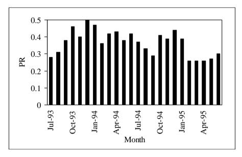
FIGURE 1: Mean monthly performance ratios of the 1.2 kWp stand-alone PV system.
