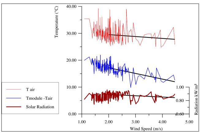
FIGURE 2: Ambient temperature, difference between ambient and *PV* module temperature and solar radiation vs. wind speeds between 11:00 and 13:00, for clear days in July and August, 1993 and 1994.
