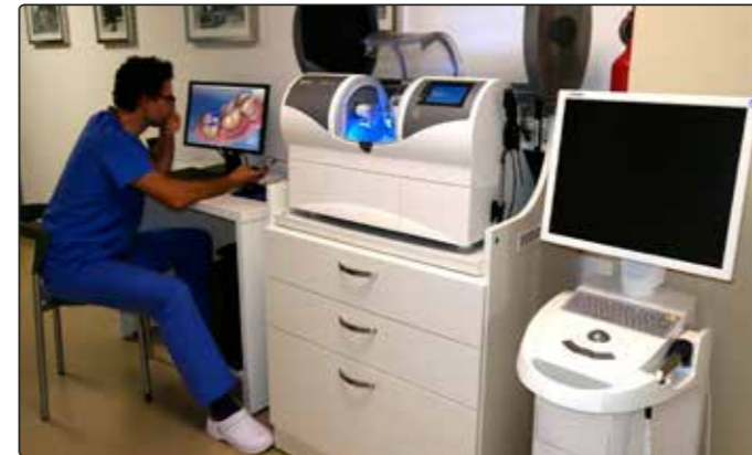
Full digital workstation of Dental and Implantology Unit at St James Hospital including acquisition unit, milling machine and secondary design computer
