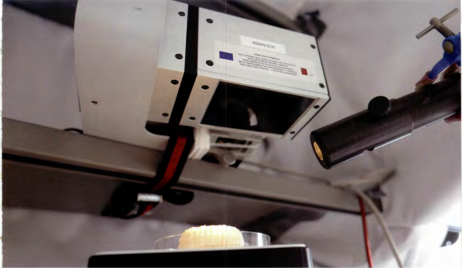
The Maltese cheeselet inspected for microbes using hyperspectral imaging Photo by Dr Sholeem Griffin
