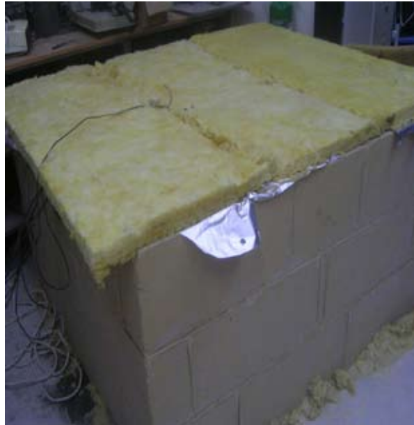
Picture 2 Insulation with aluminium foil lining
