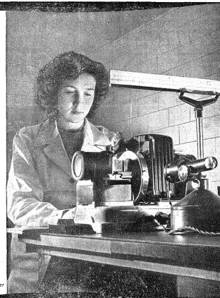
The Spekker Absorptiometer
