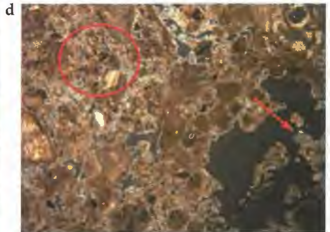
Unit 2 (PPL). Note predominance of calcitic clay (circle) and aggregates of microspartic calcium carbonate (arrow).
