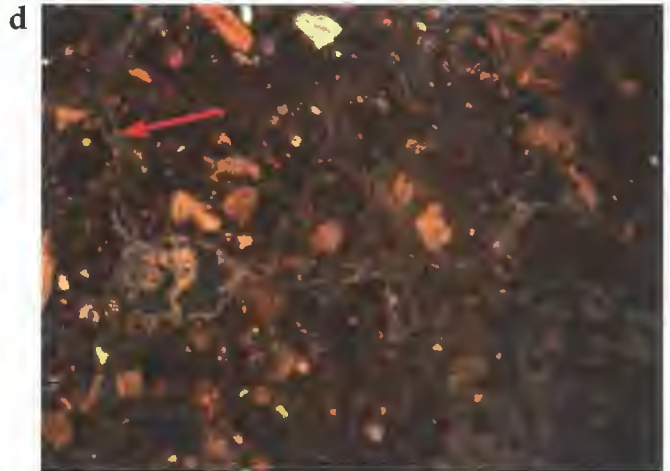
Matrix of the degrading pottery (PPL). Note the high frequency of clay and planar voids (arrow).
