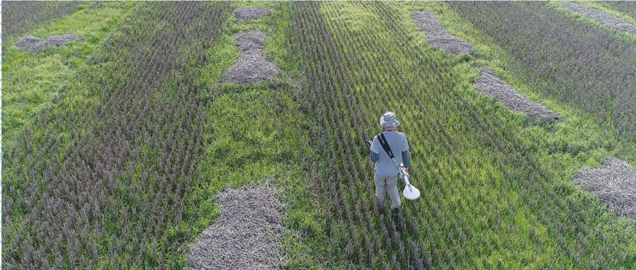
Electromagnetic induction survey along Ashberton coast
