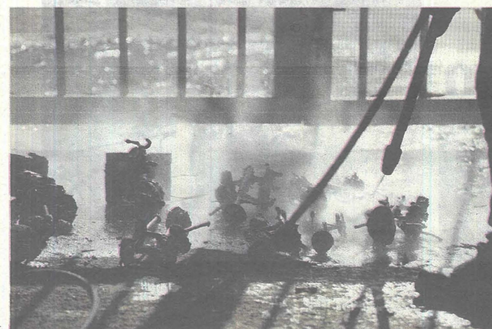
Cleaning bronzes just after the casting from residual luto.
