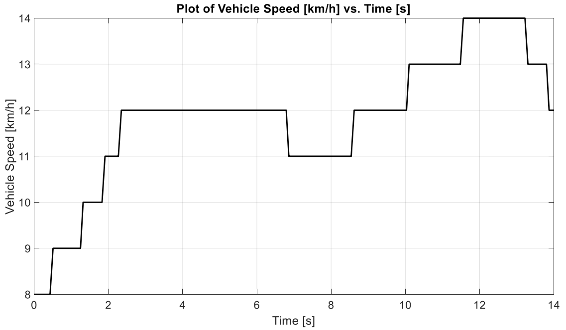
Figure 2.10 – Plot Vehicle Speed [km/h] vs. Time [s], with a vehicle speed setpoint of approx. 10 km/h and angle tilt for roundabout turn.
