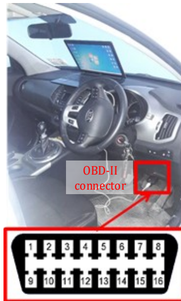
Figure 2.5 – Kia Sportage 2014 OBD-II port connection
