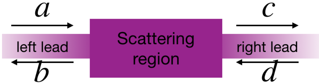
Figure 4.1: Two leads are connected through a scattering region. The four states represented as a, b, c, d travel in the two directions. The transport is calculated from the left to the right lead making use of the scattering matrix S .
