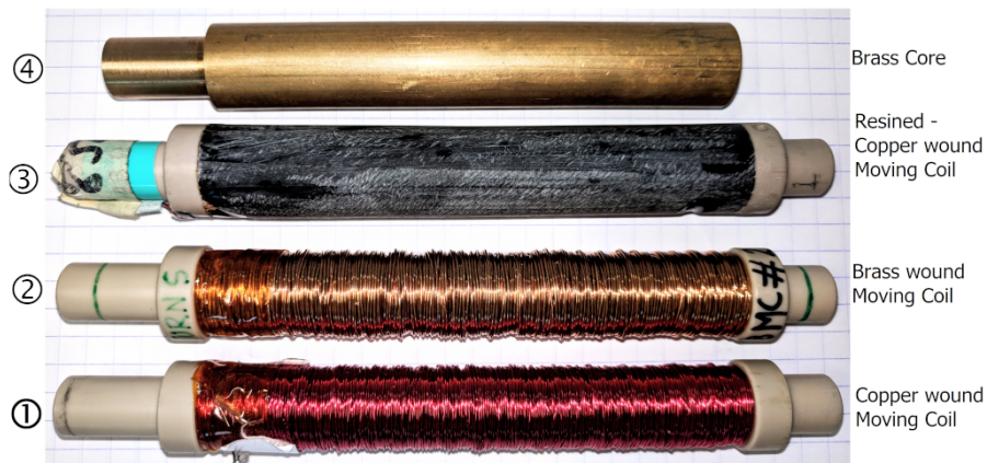
Figure 5.13: Comparison of the normal moving coil (Coil 1), the new coil made out of brass cable (Coil 2), a normal moving coil which is encased in resined (Coil 3) and a brass core (4).
