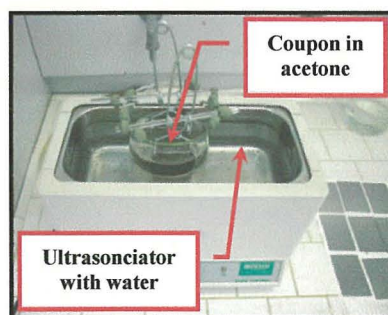
Figure 3-10 Removal of surface matter from armour analogues by ultrasonication
