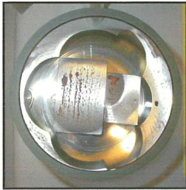
Plan detail of coupons (experimental & control) from Coupon Series 6 on sputtering stage before sputtering
