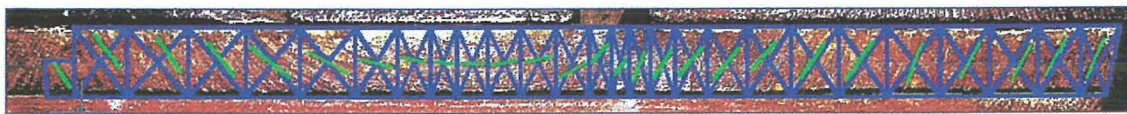
Plate 5 Board 3 showing the virtual divisions and the direction of the growth ring
