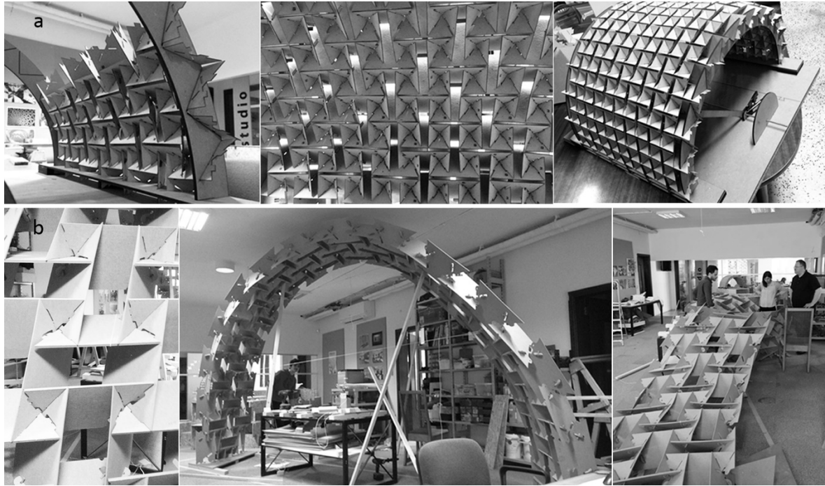
Figure 34: Test Models to Derived Based Surface Geometry a) A cardboard scale model of a barrel vault pavilion. The construction is based on fixed boundary arches, trammel, and plate configuration with nibs and slits b) Full scale prototype of three circular arches of the barrel vault pavilion in MDF. Source: Author
