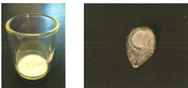
Figure D.6.1: Melted filter crucible (before and after heating at 900°C)
