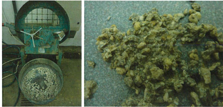
Figure 6.4: Mixing sample (greater than 4mm) in pan mixer (left) and washed material passing 4mm sieve after mixing in pan mixer (right). Photos by author (2011)
