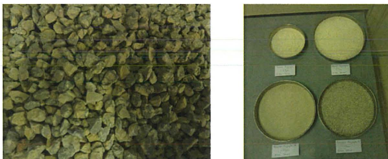
Figure 4.6: Sample preparation of bridge material for flakiness index and chemical tests A distinct visual difference can be made between natural (white) and recycled (grey) aggregate. Photos by author (2011)
