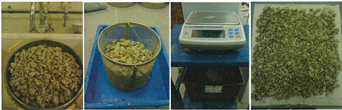
Figure 6.7: Water absorption using wire basket for all samples graded 9/18 Photo by author (2011)
