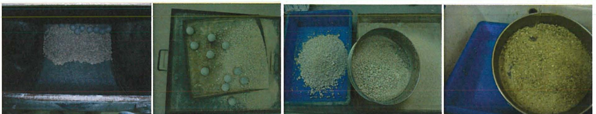
Figure 6.5: Process of LA experiment carried out on graded material of 10/14 up to wet sieving of material retained on 1.6mm sieve. Photo by author (2011)
