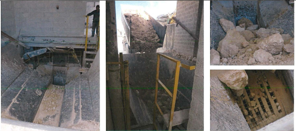
Step 3: Sieving the material into different grades (0 to 6mm, 6 to 9mm, 9 to 18mm)
