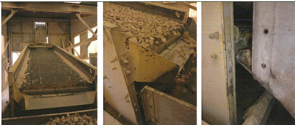
Step 3: Sieving the material into different grades (0 to 6mm, 6 to 9mm, 9 to 18mm)
