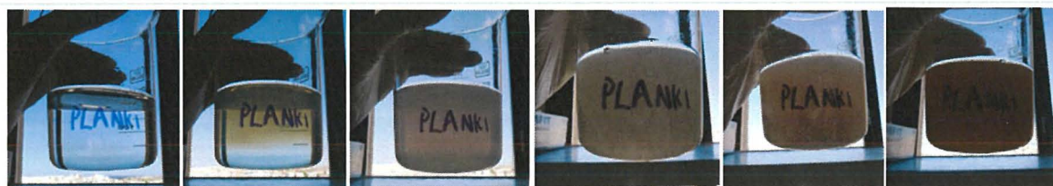
Figure 6.17b: Photos showing gradual change in colour from clear filtrate to opaqueness up to finally the overshoot of the limit with a permanent brown trace. The limit (recorded result) is easily detected since the brown trace on the white colour is very distinct (fourth to fifth photo below).
