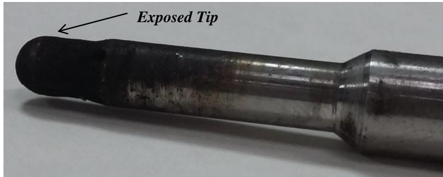
Figure 4.47. The in-cylinder pressure sensor showing signs of soot at the tip.
