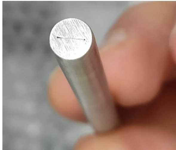
Figure 5.10. The surface of the Aluminium eroding thermocouple.
