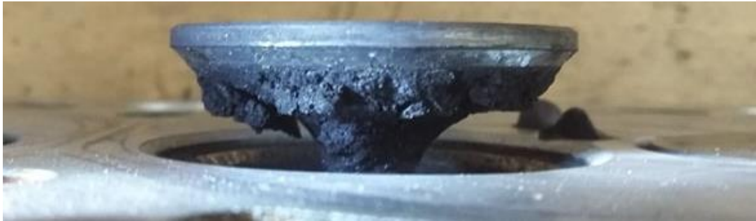
Figure 3.8: Soot present on intake valve, cylinder two.
