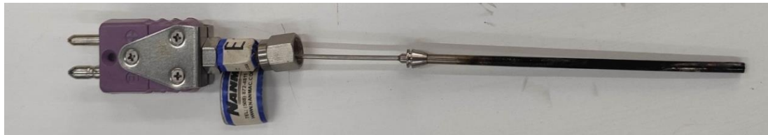
Figure 5.9. The Zirconia eroding thermocouple.
