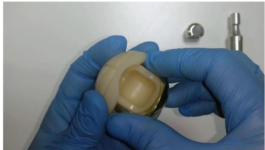
(h) Step 8: The flexor-rotator subassembly is inserted inside the MaltaHip cup.
