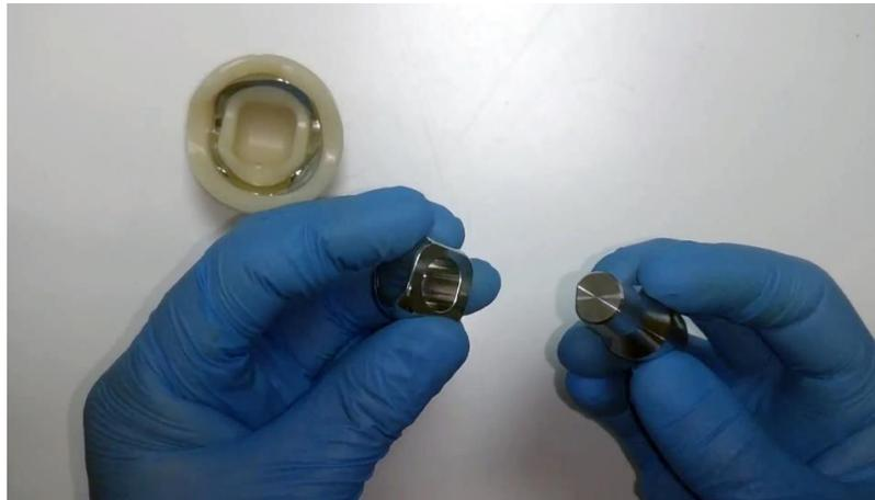
(k) Step 11: Due to the orientation-dependency of the design, a flat surface has been incorporated which act as a key for aligning the components.
