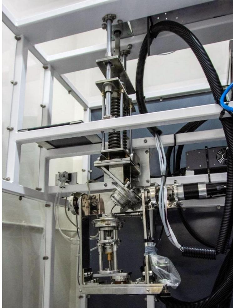
Fig. 3.21: In-house developed hip joint simulator. Flexible enclosure which contains the fluid during testing is not shown in the photo.
