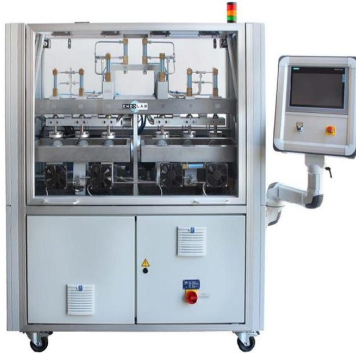
Fig. 3.23: Endolab® Mechanical Engineering GmbH six-station hip joint simulator according to ISO 14242-1:2014/Amd 1:2018. Source: Endolab® report (unpublished).
