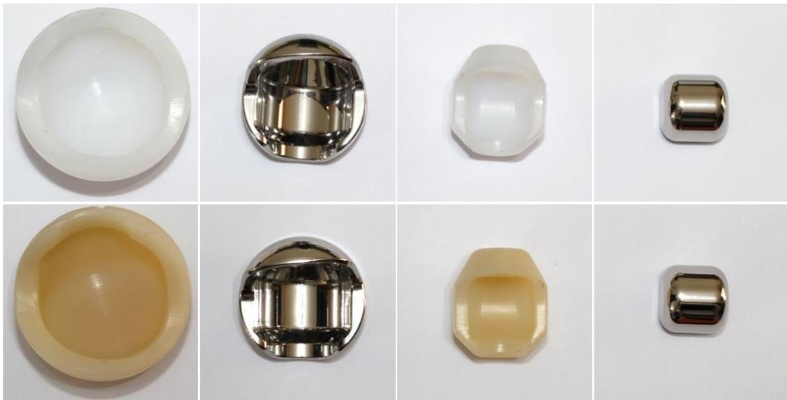
(a) The components of the MaltaHip with two different polymeric materials: UHMWPE (top) and VEHXPE (bottom).
