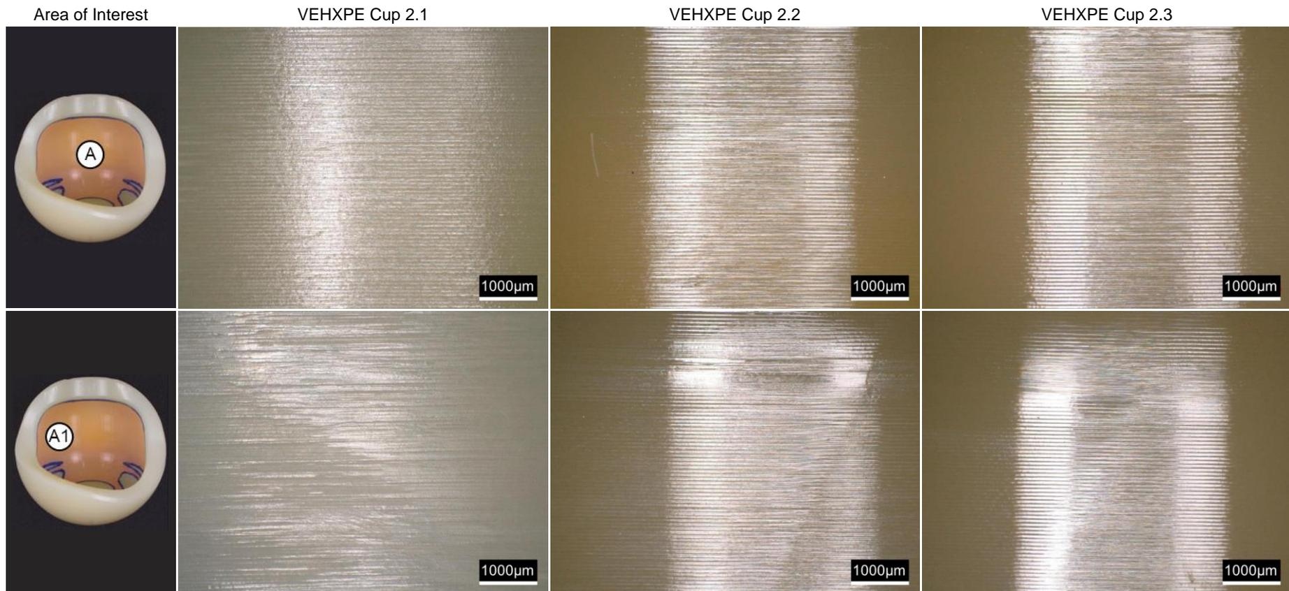
Fig. 5.107: Microscopic images of the MaltaHip VEHXPE cup at the internal superior surface. Results produced by Endolab®.
