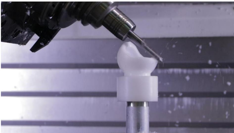
(c) Close-up of the outer edge profile being machined.
