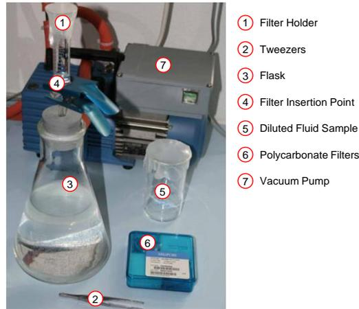
Fig. 3.26: Filtration system used for the particle analysis preparation according to ISO 17853:2011. Source: Endolab® report (unpublished).
