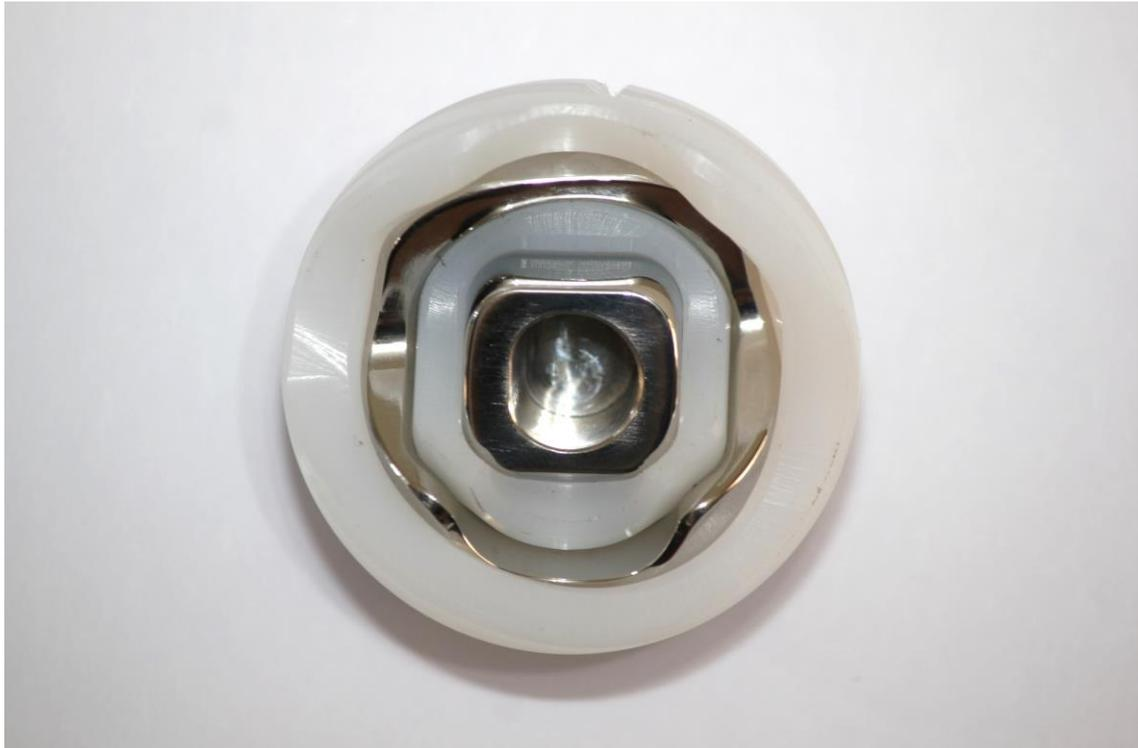
(a) The components of the MaltaHip produced out of high-N austenitic stainless steel and UHMWPE components.
