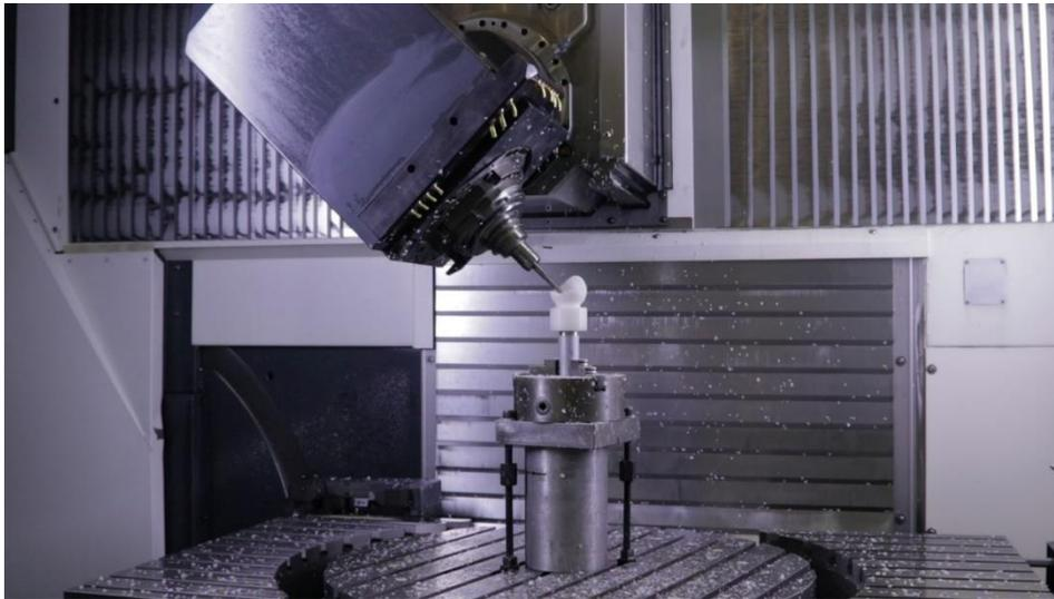
(b) Machining of the MaltaHip cup using the swarf milling technique.
