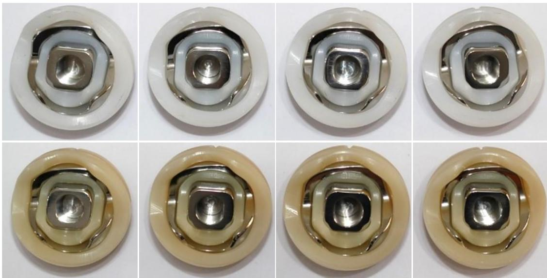
(b) The eight implants that were tested at Endolab: UHMWPE (top) and VEHXPE (bottom).
