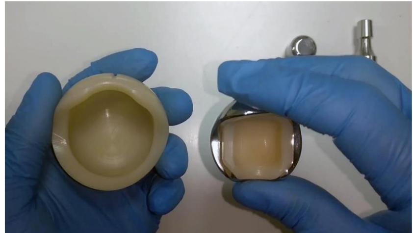
(f) Step 6: The next step is to engage the flexor-rotator subassembly inside the MaltaHip cup.
