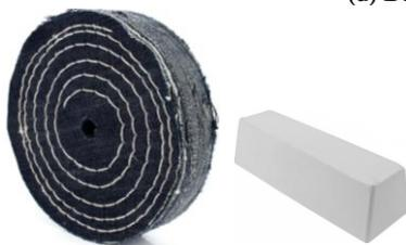
(b) First stage (roughing) polishing procedure. Source: [321].
