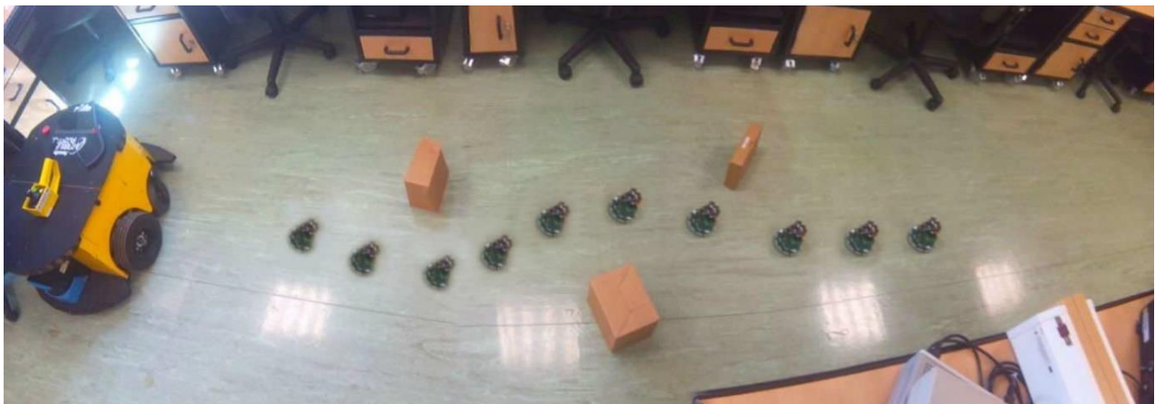
Path taken by Khepera III while approaching a target (the yellow robot on the left)
