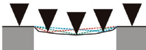
Figure 2.13: Schematic of the AFM tip at different positions on the sample; the dashed lines represent the shape of the membrane at the corresponding contact point, the solid line represents the acquired tip trajectory and thus the obtained AFM topography image [135].
