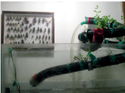
Figure 2.2: The eco-purifier set up in a 40-litre aquarium
