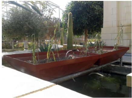
Figure 2.1: The eco-purifier set up in a 65,000-litre pond measuring approximately 4mX2mX1m
