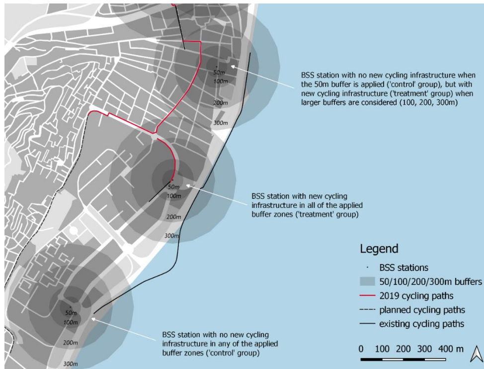
Figure 8.5: Comparison of different buffers around BSS stations in Las Palmas de Gran Canaria
