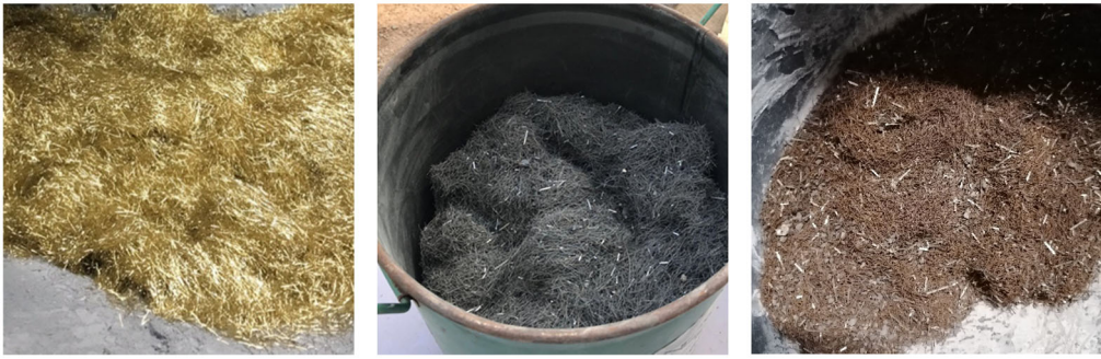
Figure 6. Original fibres (left), fibres separated at the recycling plant (middle) and fibres separated from the aggregates at the laboratory (right).
