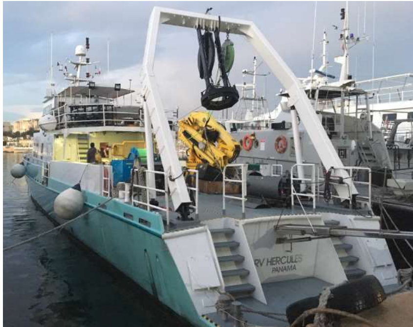
Figure 6: Winch (blue with green cable) and winch block (green) on A-frame. The winch was welded onto the deck.
