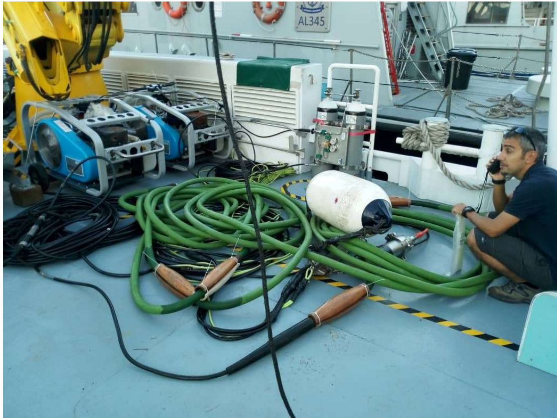
Figure 15: The seismic reflection profiling setup laid out on deck. Shown in the photos are the air gun, streamer and compressors.
