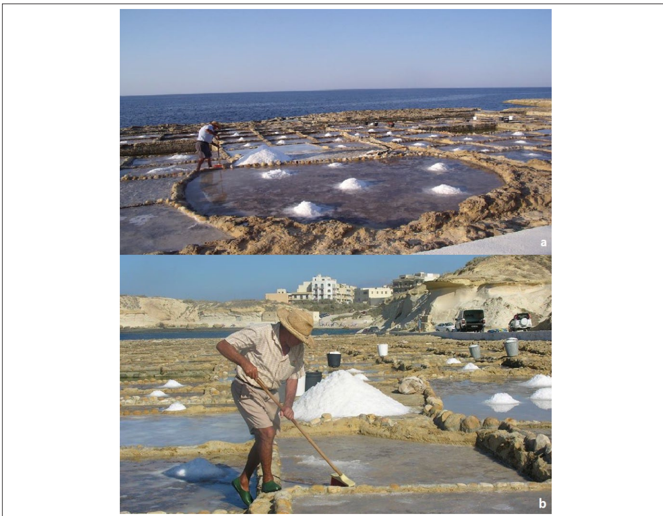
Figure 4. (a) Located strategically on the foreshore, the rectangular crystallizers occupy significant areas near the shoreline at Xwejni Bay (Gozo), and (b) the salt is collected manually by Emmanuel Ċini in single heaps and then transferred to larger collection pans to drain from excess seawater fluid for another week.
