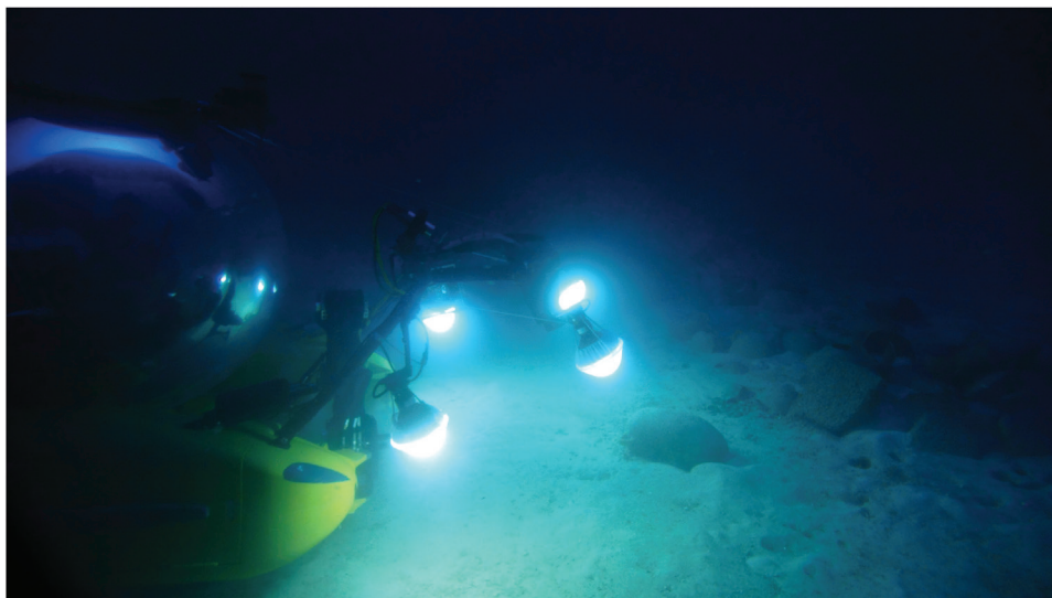
Fig 9: The trifocal system mounted on the REMORA 2000
