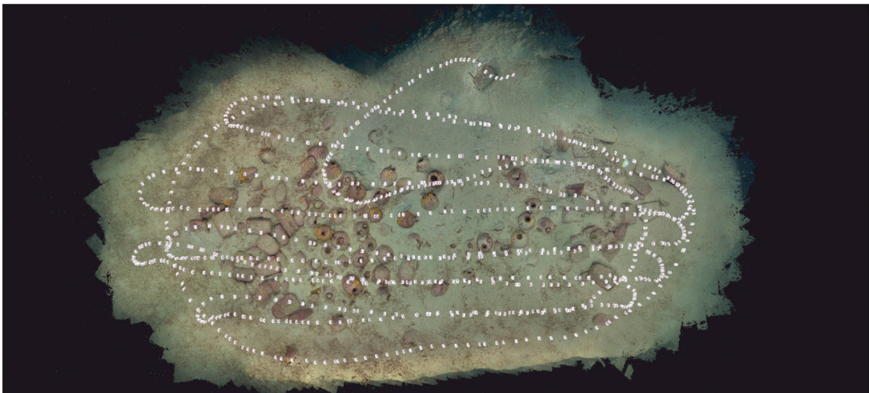
Fig 13: An example of swim lines undertaken by underwater cameraman for the acquisition of video footage for the production of the photogrammetric model
