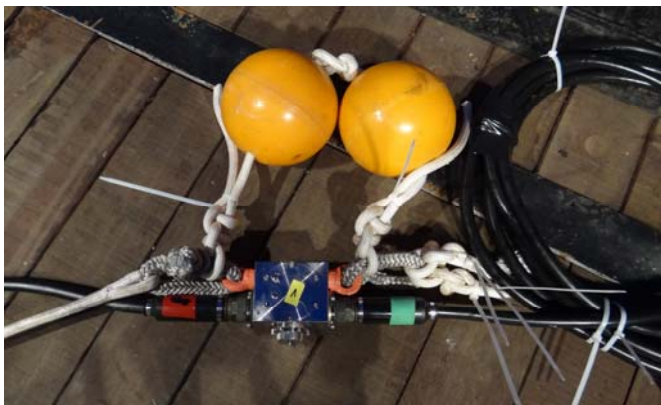
Fig. 22 Floats are fixed on the cross cable in order to keep it at about 2 m depth during profiling.
