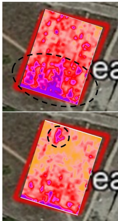
Figure 5. Depth slices in Area 3 (600 MHz). ( Upper panel ): 10 ns (60 cm). ( Lower panel ): 15 ns (90 cm).
