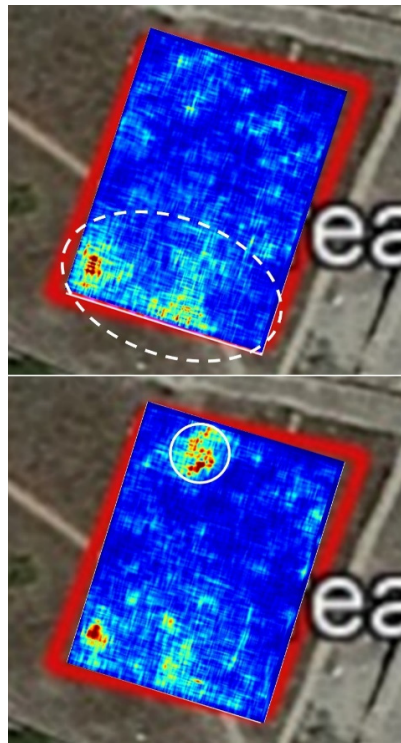
Figure 9. Depth slices in Area 3 (600 MHz) achieved with an inverse scattering algorithm. (Upper panel): 75 cm. (Lower panel): 110 cm.
