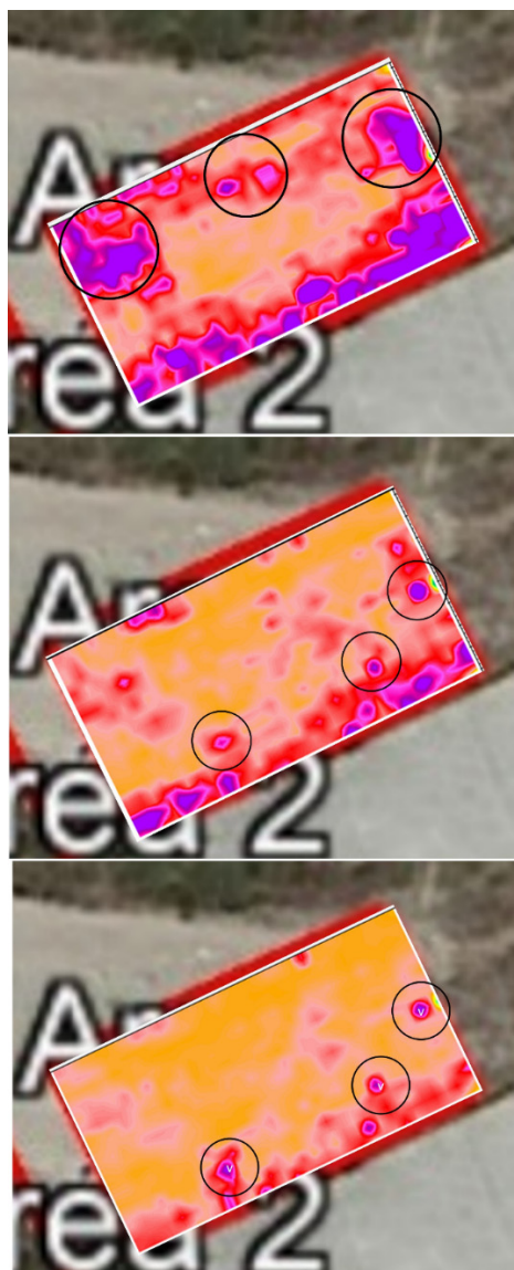
Figure 3. Depth slices in Area 1 (600 MHz). ( Upper panel ): 5 ns (28 cm). ( Middle panel ): 10 ns (55 cm). ( Lower panel ): 15 ns (83 cm).
