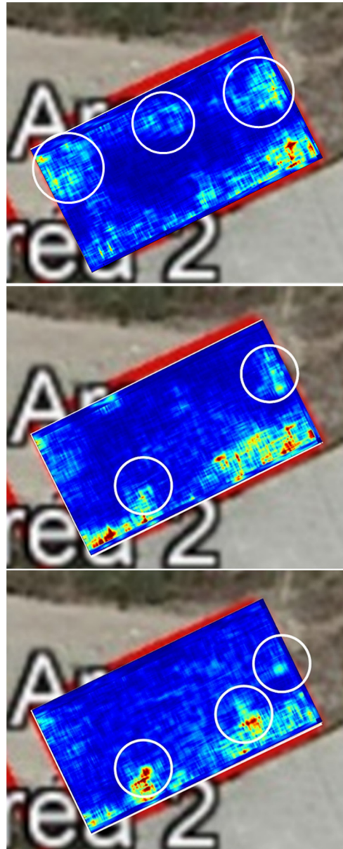
Figure 7. Depth slices in Area 1 (600 MHz) achieved with an inverse scattering algorithm. ( Upper panel ): 40 cm. ( Middle panel ): 75 cm. ( Lower panel ): 102 cm.
