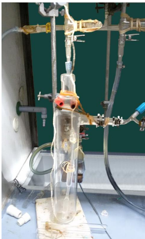
Figure A-1.9: Large tube-like flask set up used to purge and fill ampoule tubes.
