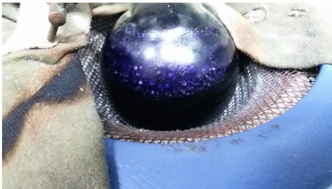
Figure A-2.2: Toluene being dried in still showing typical deep purple colour of Na/Benzophenone indicator indicating dryness
