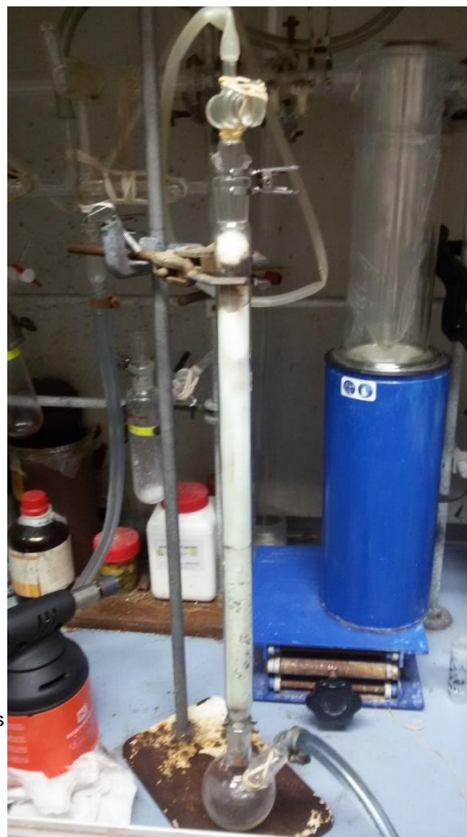
Figure A-1.1: Set up for the reduction of \text{MnO}_2 to \text{MnO} oxygen scavenger, diagram (left, drawn using ACD/ChemSketch software) and photograph (right).
