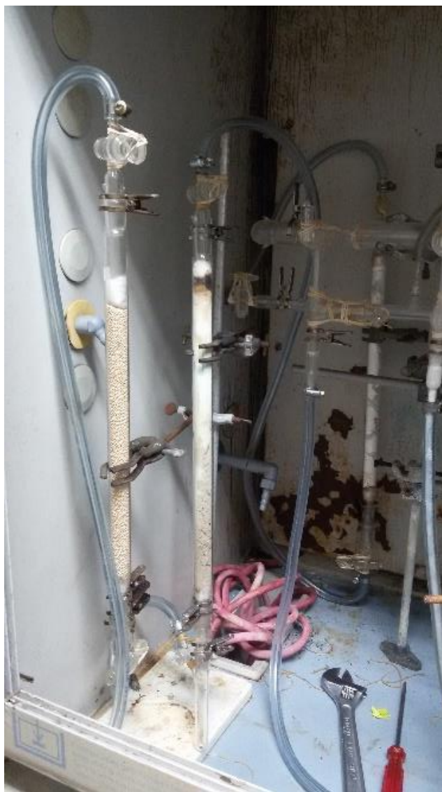
Figure A-1.2: MnO column set in line in the path leading argon to the Schlenk line.
