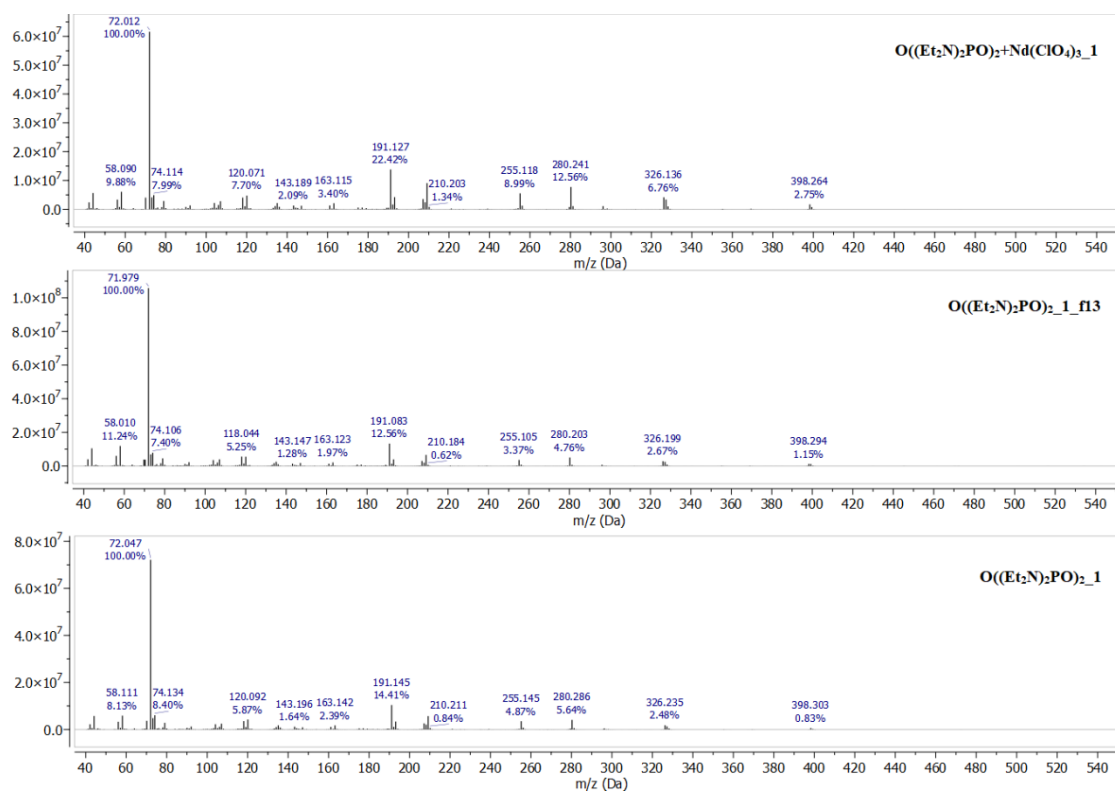
Figure 4.128: Comparison of the Mass spectra of O((Et_2N)_2PO)_2_1 (GC peak at 10.90 min.), O((Et_2N)_2PO)_2_1_{f13} (GC peak at 10.56 min.) and O((Et_2N)_2PO)_2_1 (GC peak at 10.60 min.).
