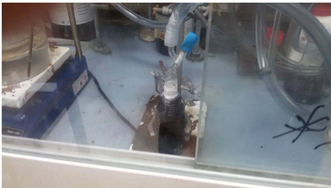
Figure A-4.4: Purging of amber glass bottle to be used for the storage of PPTC.
