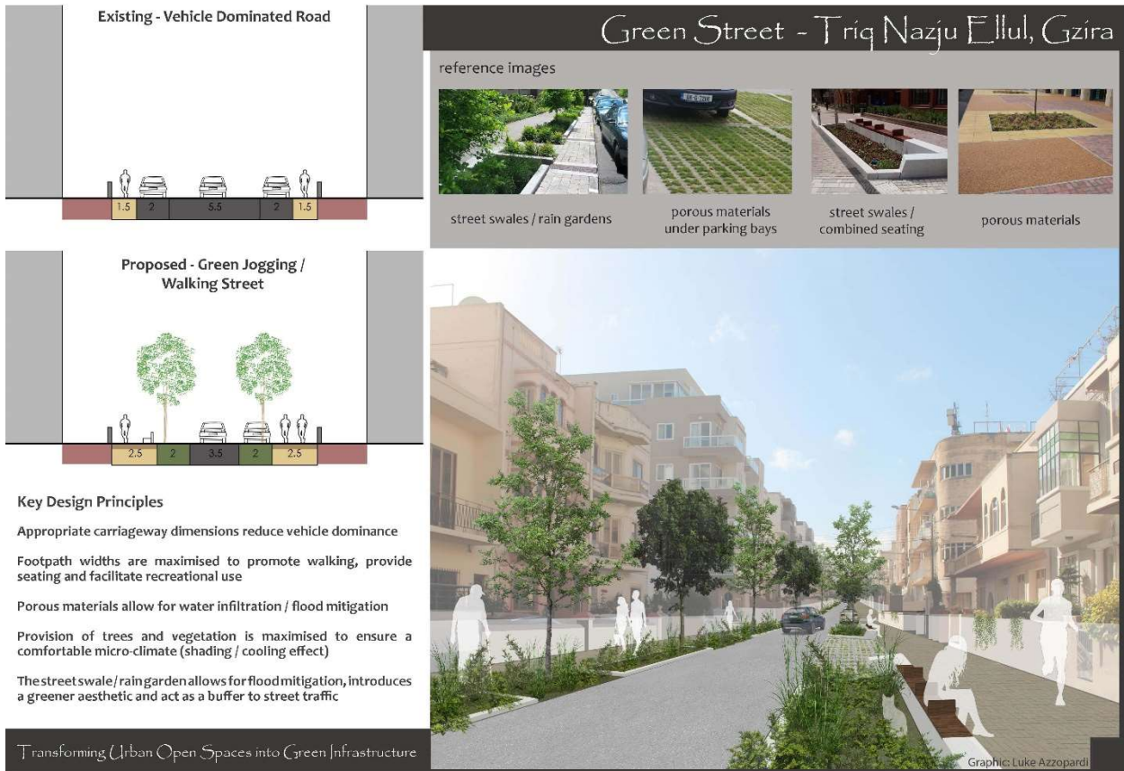
Figure 160: Illustrating the potential for a 'green' street
