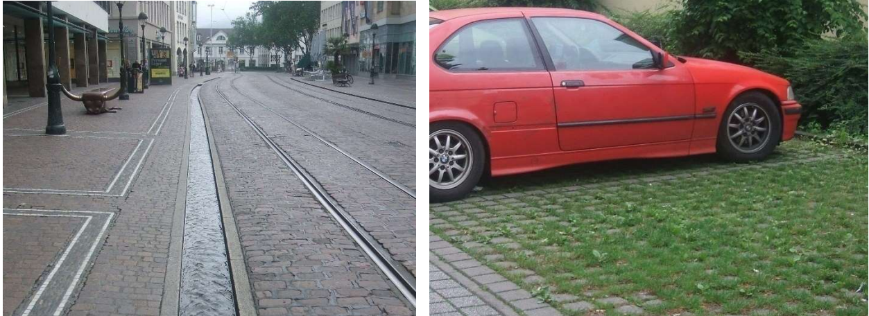
Figure 17: Exposed water channels and permeable surface areas in Freiburg
