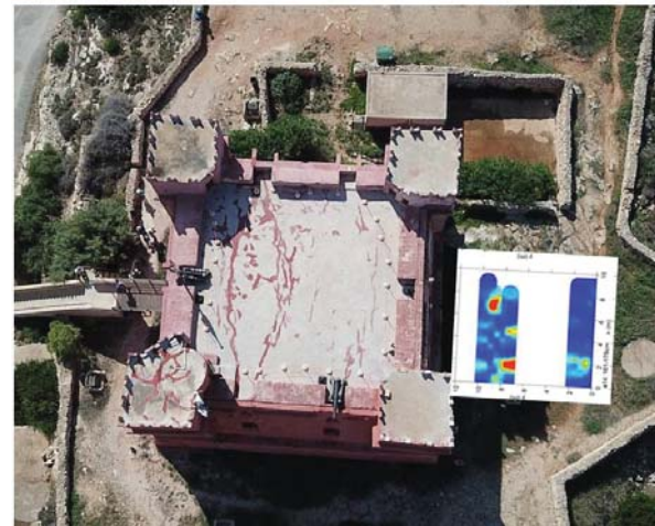
Fig. 3. GPR slices close to the Red Tower. On the GPR slices close to the Red Tower. At the top: depth of about 70 cm. At the bottom: depth of about 100 cm
