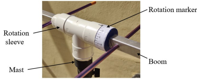
Figure 4.19: Rotating mechanism for reference antenna
