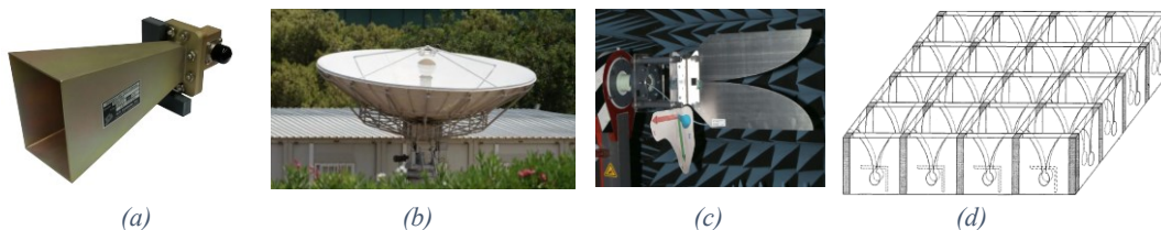
Figure 2.27: Aperture Antennas (a) AH Systems SAS-584 Horn Antenna 5.85GHz – 8.20 GHz [130] (b) radio telescope reflector antenna at the University of Malta (c) Vivaldi antenna [131] (d) Egg-crate structure [132]
