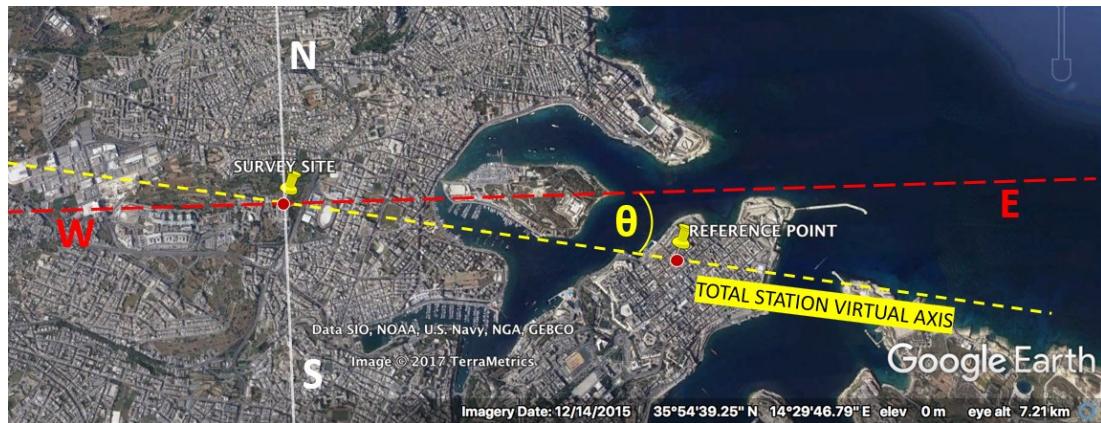
Figure 3.3: Virtual axis reference for Total Station reading calculations
