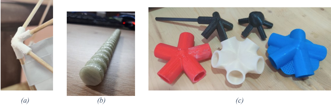
Figure 3.25: (a) GFRP threaded rod (b) prototypes of matching vertex joints: (b) short rod support version with flat vertex (c) webbed and long rod support versions
