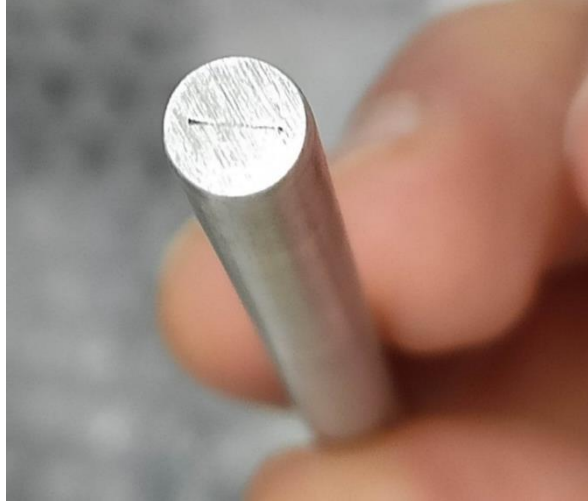
Figure 5.10. The surface of the Aluminium eroding thermocouple.
