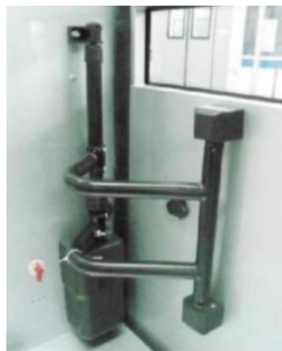
Figure 2.2: The electrical drive used to operate the sliding doors [26].
