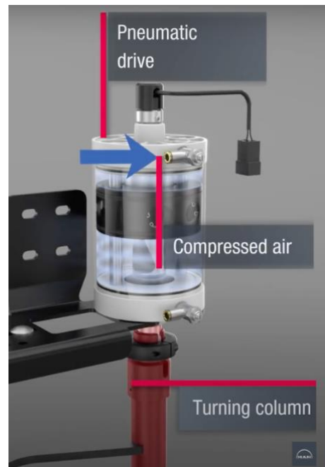
Figure 2.8: Newly developed pneumatic door motors by MAN [46].
