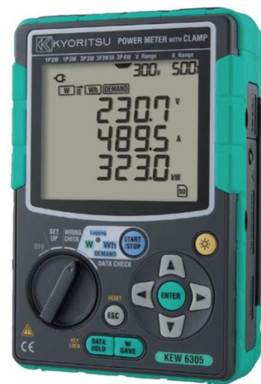
Figure 3.8: The Kyoritsu KEW 6305 Power Meter [75].
