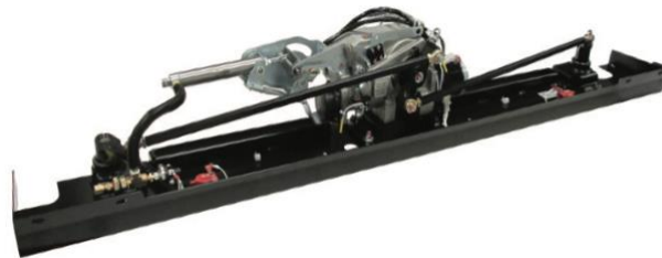
Figure 3.12: The electromechanical motor used for the conversion of the pneumatic cylinders [95].
