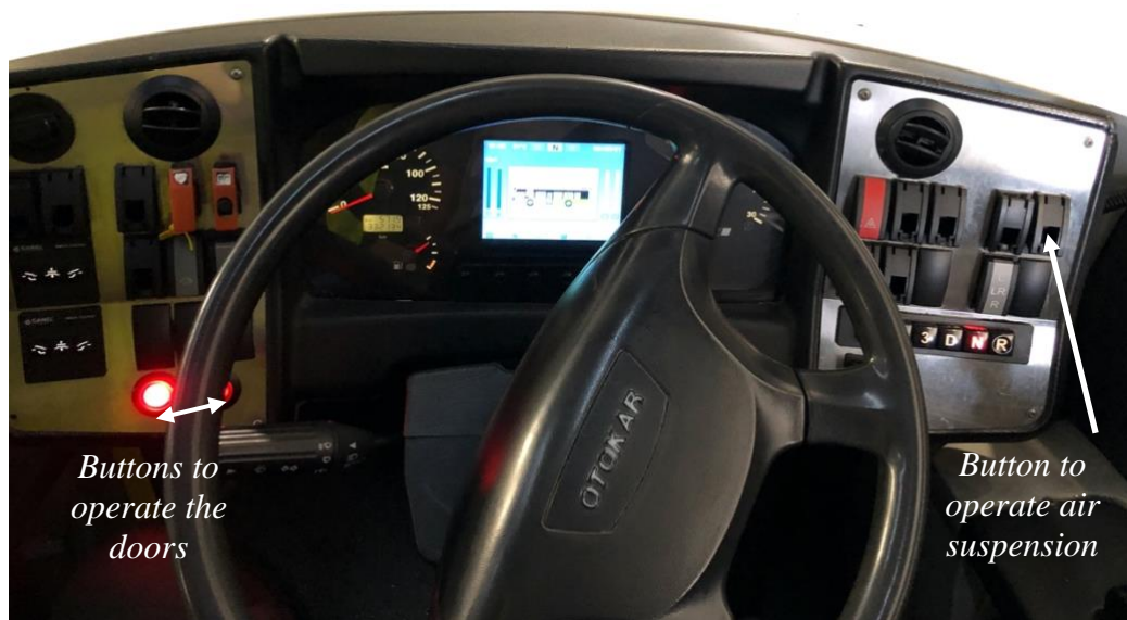
Figure 6.3: The buttons used to operate the auxiliaries.
