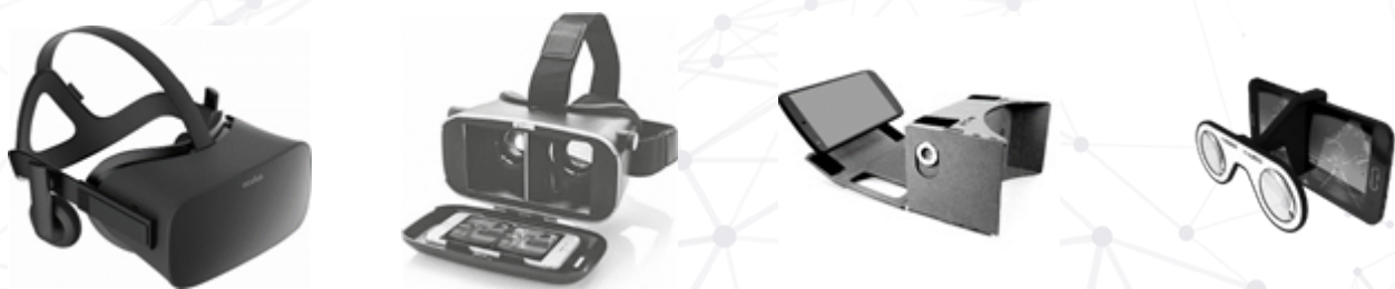
Figure 37: Examples of a headset, polyester insert VR glass, cardboard insert VR glass, and click-on VR class.
