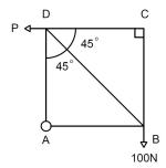
The framework lies in a vertical plane with DC above AB, both rods being horizontal. The framework is smoothly hinged to a fixed support at A, and carries a vertical load of 100 N at B. The system is held in equilibrium by a horizontal force P at D.
