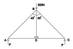
The framework lies in a vertical plane, and rests with ADC horizontal on two supports at A and C. The framework carries a load of 300 N at B. Find:
