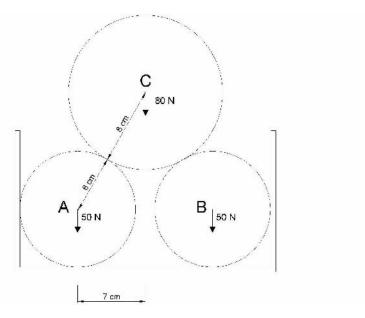
Cylinders A and B, which are identical, each having weight 50 N and radius 6 cm, lie against the sides and on the base of the gutter. Cylinder C, which rests on top of A and B, has a weight of 80 N and radius 8 cm. The distance between the centres of A and B is 14 cm. Find:
