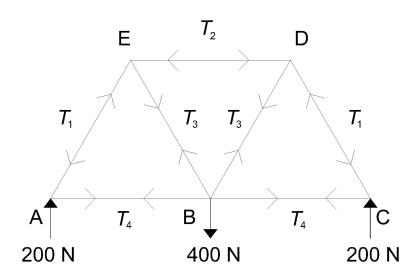
Find the forces in the rods, stating whether they are in tension or in compression.
