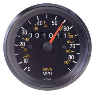
The picture shows the speedometer of a car with an outer scale showing miles per hour and an inner scale showing km per hour.
