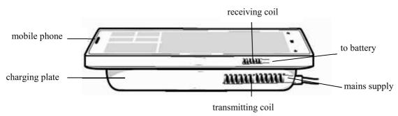
Wireless charging is a popular new feature included on some mobile phones. The phone is placed on the charging plate and the phone charges wirelessly. The diagram above shows a charging plate which has a transmitting coil connected to a mains supply and a mobile phone. Inside the mobile phone there is a receiving coil which is connected to a battery.
