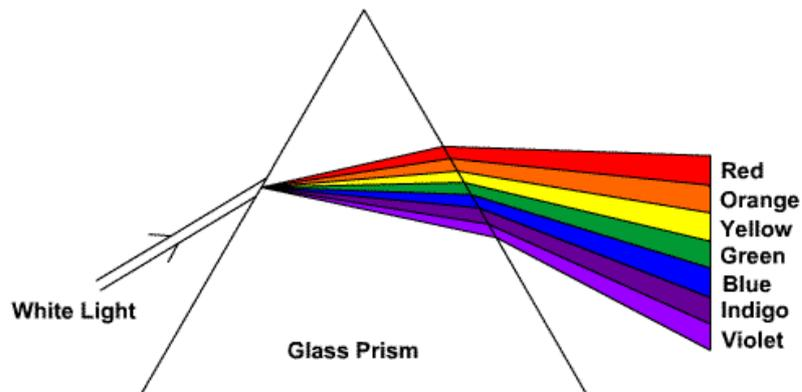
a. White light is made up of different colours. Dispersion occurs when a ray of white light passes through a glass prism.
