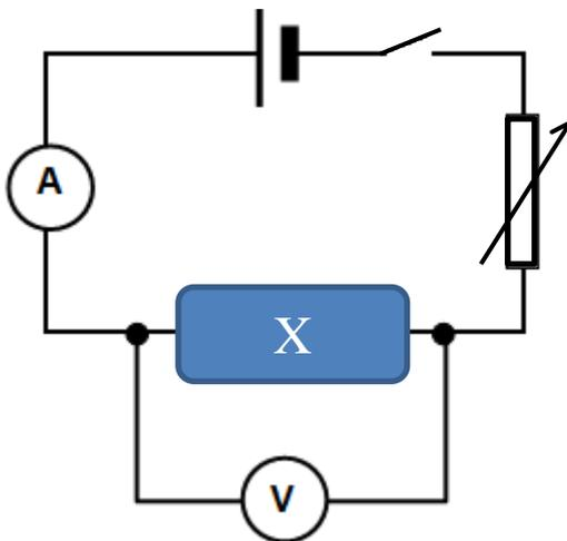
For different settings of the variable resistor, the following data was recorded:
