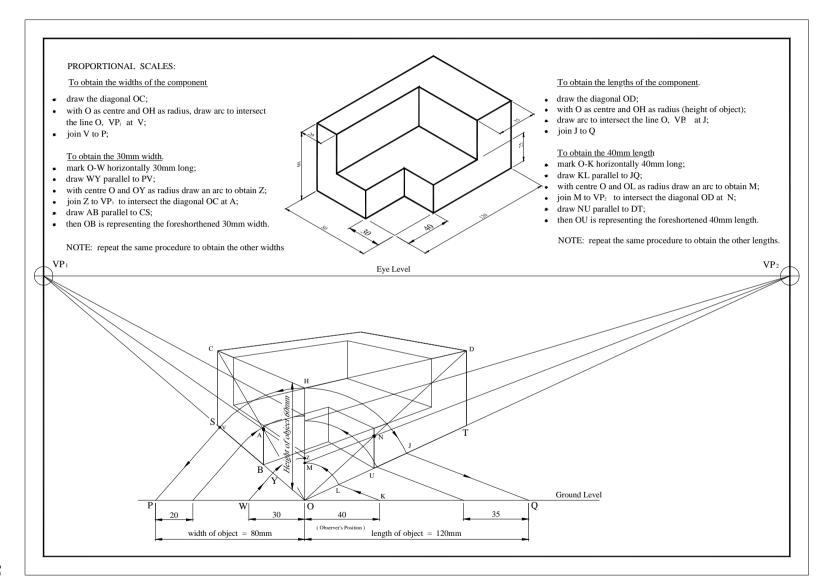
Worked example of a two point perspective view (alternative method)
