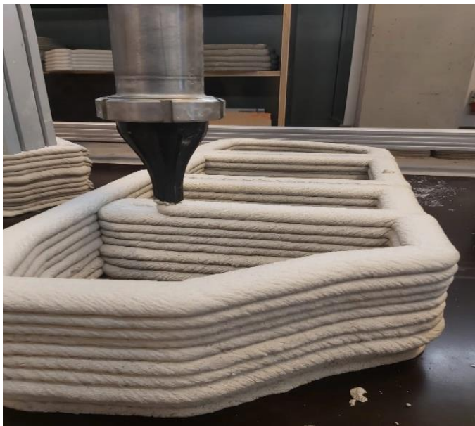
Fig. 6. 3D printing of ternary GCP composition.
