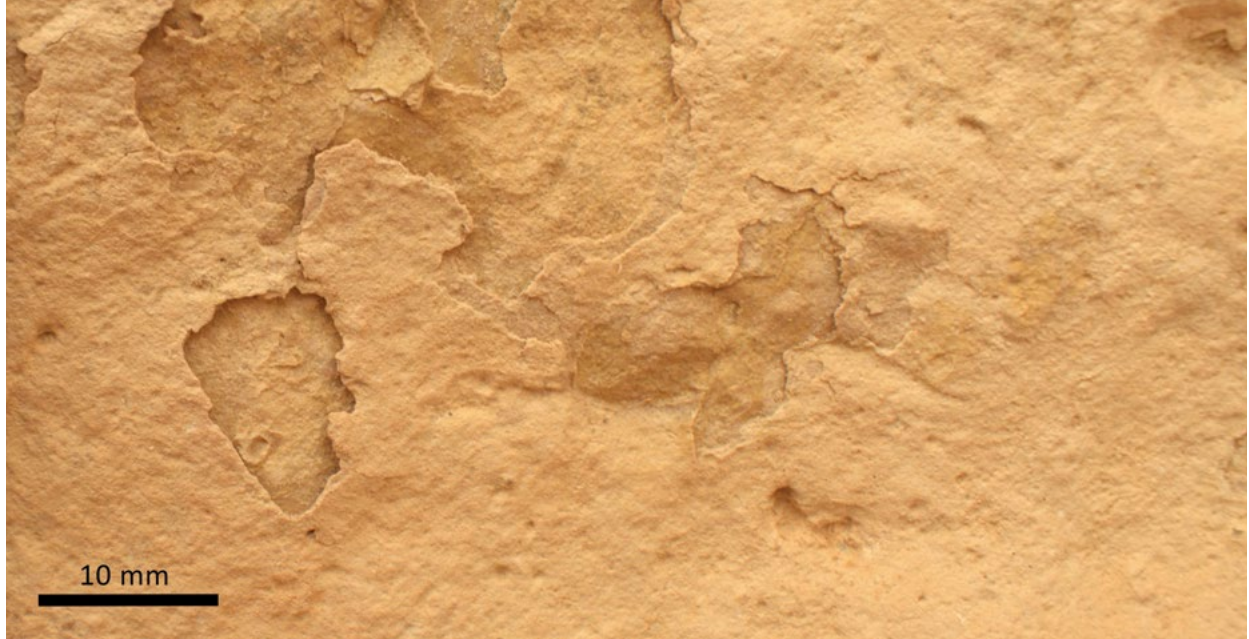
Detail of stone flaking at the Megalithic Site of Mnajdra, macro photo Photo by Rosangela Faieta
