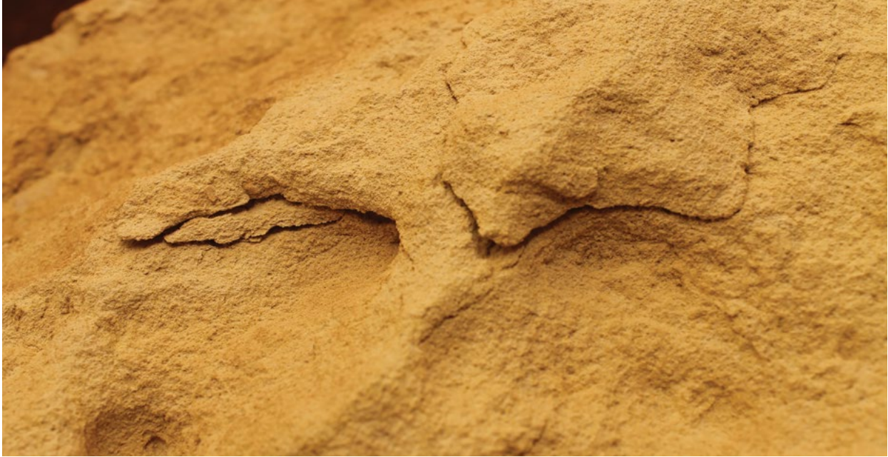
Evidence of stone scaling on the surface of Globigerina Limestone Photo by Rosangela Faieta
