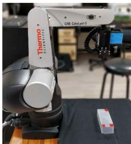
Figure 3.3: The eye-in-hand visual servoing system
