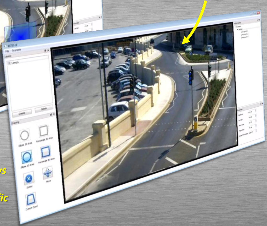
Traffic light lamp layer – detects the true current status of the lights
