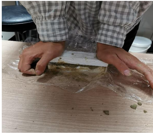
Figure 4: The two parts of the moulds are covered with plastic film and the clay is pressed.
